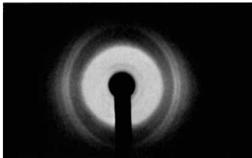
Fig. 4.—Weissenberg X-ray diffraction photograph of nylon 66.
