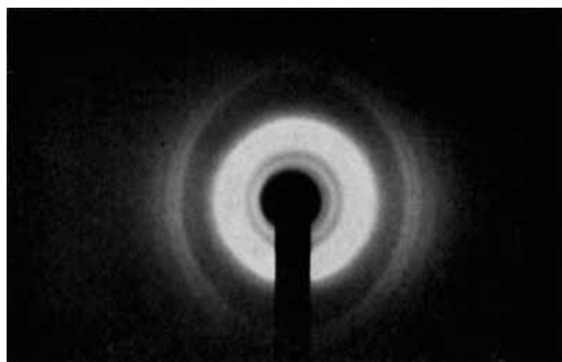
Fig. 3.—Weissenberg X-ray diffraction photograph of nylon 66 treated with sorbic acid.
