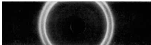
Fig. 1.—Debye-Scherrer X-ray diffraction photograph of nylon 66 treated with sorbic acid.
